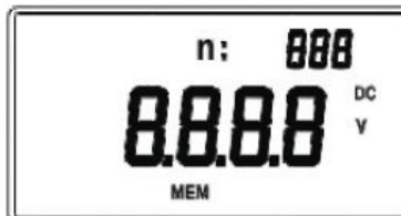
Press MEM button to page down, and press Shift button to page up; press MEM button longer than 1S, then the secondary screen display the key remain time.when the key remain time is zero,the meter will be back to Record status.
