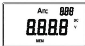
Press MEM button ,the secondary screen display the sequence number of the recorded value and the Primary display corresponding value.
