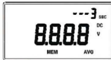
When the remain key time is zero ,the secondary screen display the counts of the recorded value as follows
