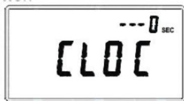
The meter enter timer set-up status, the secondary screen display the preset time
