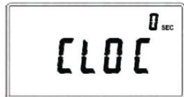
Press HOLD button will save measuring time, and exit the assign status.
