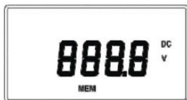
In recording status, press MEM button in succession, the meter will display the Max value, Min value, and Avg value.
